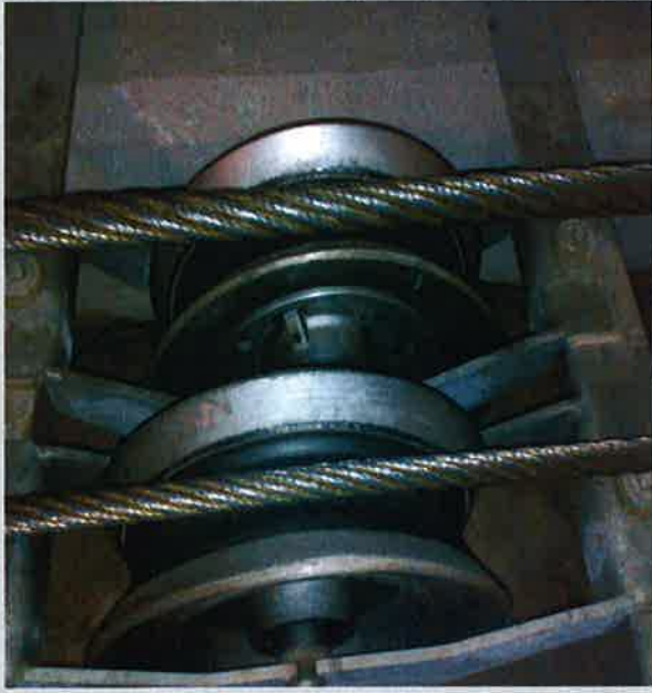
Haul rope vibrates laterally hitting line-sheave side flanges repeatedly
