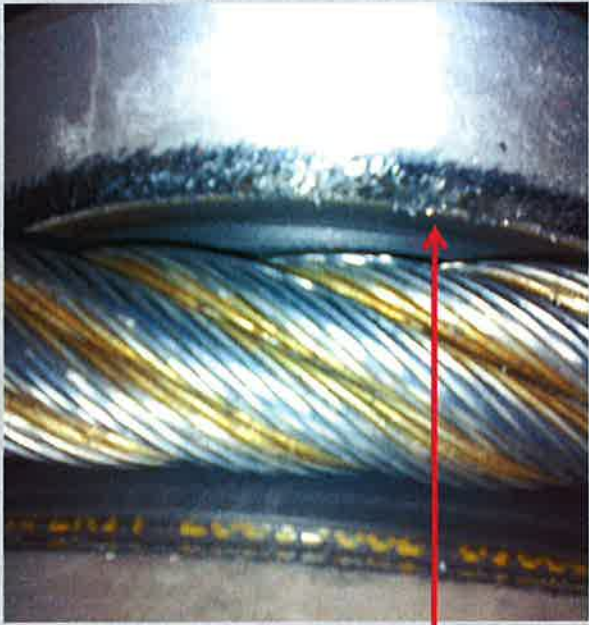
Haul rope vibrates laterally hitting line-sheave side flanges repeatedly
